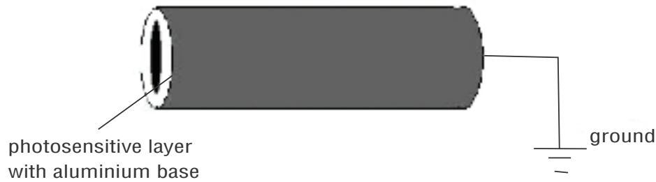
Fig. 13 Photosensitive Drum with aluminium base
